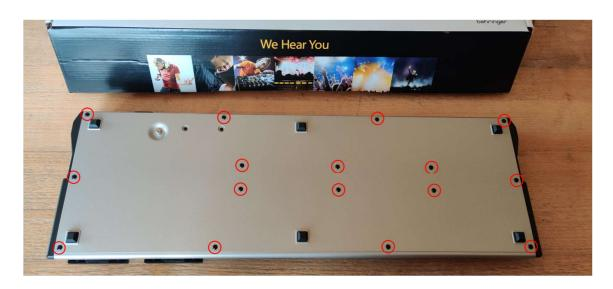
Turn the FCB1010 upside down, remove 16 screws to open the housing, lay the bottom plate next to the housing (leave the ground wire connected)
