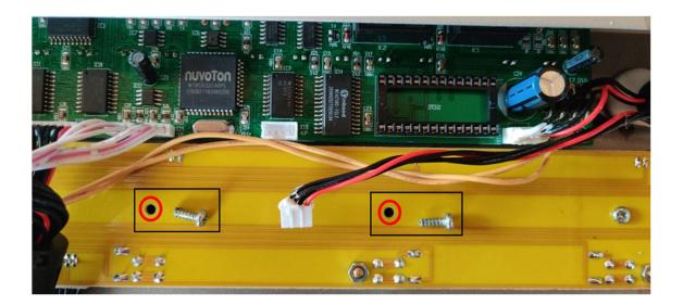
Reuse the 2 screws to mount the WIFI module. The module orientation is so that the 4-pins connector is close to the now empty 4-pins connector on the FCB1010 main board. Plug the large red/black wire into the connector of the WIFI module, and plug the short wire unit of the WIFI module into the 4-pins connector of the main board :
